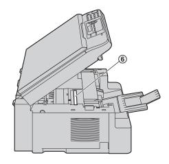
**5** Reinstall the drum and toner unit (⑦) by holding the tabs.
